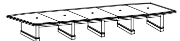
20' Boat Shaped Expandable Conference Table 713_-240EX 240W 48D 30H Consists of: -9031 Left & Right Tops -9032 Center Top & Rails (3 needed) -9033 Bases (5 needed) -9035 Rail Set for -9031 (2 needed)
